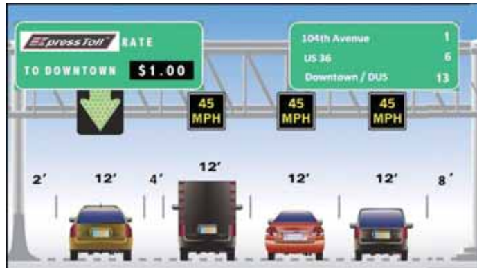
The project will implement dynamically priced managed lanes and Active Traffic Demand Management.
